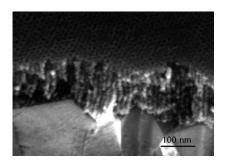
Available vacancies: Novel mesoporous titania thin films can be prepared with highly ordered vertical channels. Most of the pores are accessible from the film surface, and these channels can be filled with gold to produce gold nanowires.
